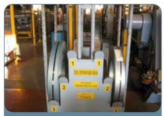
Figure 2: A rack used for separating narrow coils
